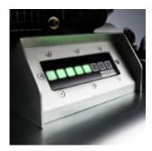
Easy to read Compatec helps the operator determine when maximum compaction has been reached. The number of lights will increase with each pass and no longer increase once maximum compaction is achieved.
